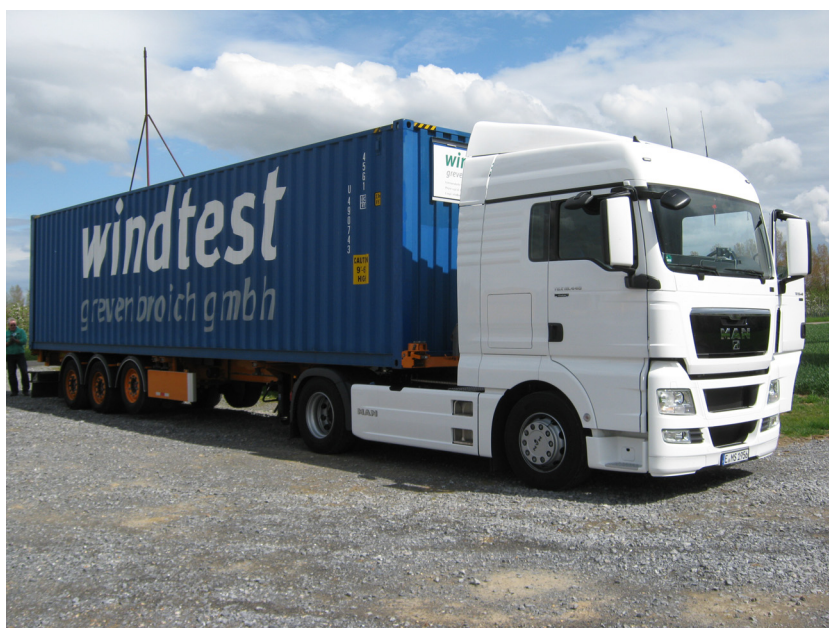
One of our LVRT containers (testing possibilities up to 6 MW)
