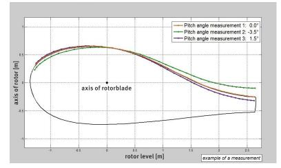
A comparison of the profile cut CAD-Data provided by the manufacturer and the three laser scanned surfaces of the blades.
